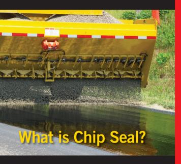
Chip seal is an application of asphalt bitumen over a prepared surface covered by a thin layer of aggregate. The many differences are that the bitumen can either be an MC (medium cure asphalt) or an emulsion (asphalt made by milling with water). Both are good products. There can also be a variation of the aggregate from pea gravel, steel slag, or a limestone chip (which is the most common used aggregate in this area).
